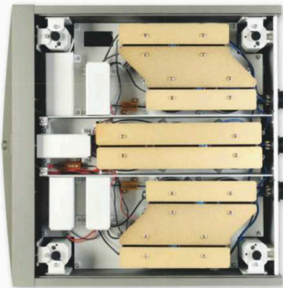
ABOVE: Supply unit includes three AC mains transformers/three banks of electrolytics for the IR LED PSU [centre] and Eq PSUs [top/bottom]
