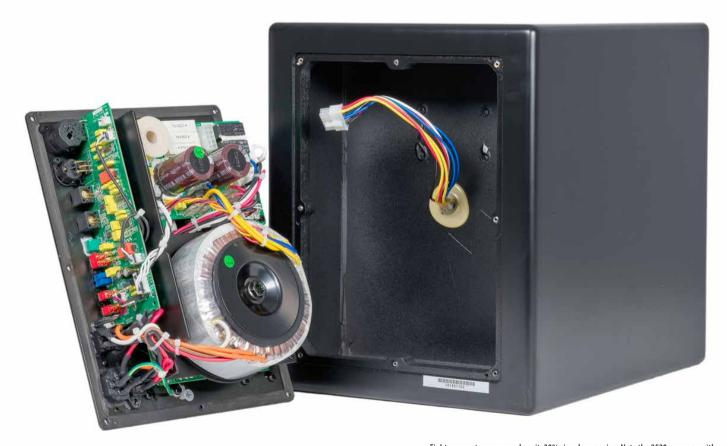
Eighty percent power-supply unit, 20% signal processing: Note the 2520s manage without any DSP. This is a rare feature among today's active speakers. Another nice design detail is the partition walls between the power supply and the signal circuit boards. You would be hard pressed to achieve a greater sense of harmony in such a small space.
