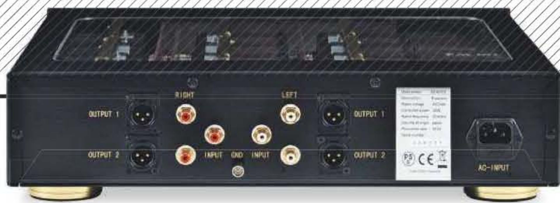
ABOVE: Rear view of the 'DS-W2 EQ' PSU/equaliser. The pick-up's internal LED is powered via the R- and L- pins while the output is returned via R+ and L+, all via the 'Input' RCAs seen here. The equalised output is on pairs of RCAs and balanced XLRs
