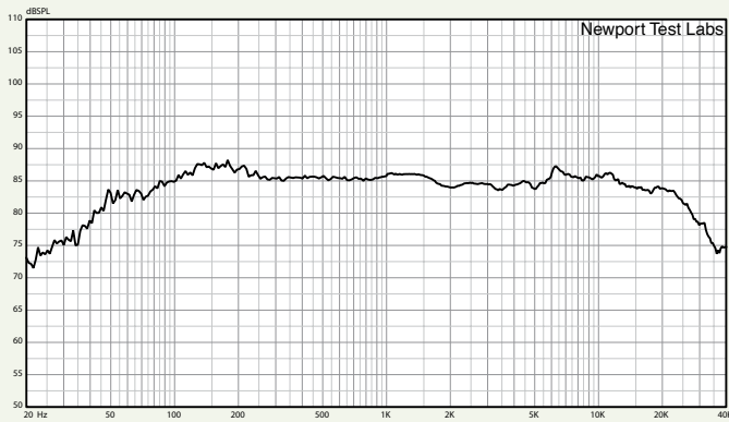
Graph 1. Frequency response. Trace below 900Hz is the averaged result of nine individual frequency sweeps measured at three metres, with the central grid point on-axis with the tweeter using pink noise test stimulus with capture unsmoothed. This has been manually spliced (at 900Hz) to the gated high-frequency response, an expanded view of which is shown in Graph 2.
