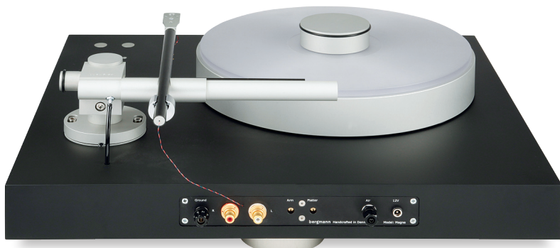
ABOVE: Rear panel connections are for ground, audio outputs and air inlet from the pump. In the centre are the two small screw adjusters for air pressure
